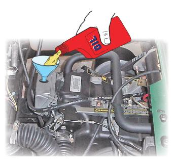
As a final check, check the oil level again with the vehicle on level ground. Like all liquids, oil increases in volume when warm. The full 'H' mark on the dipstick is calibrated for an engine at operating temperature. When the engine is cold, the oil will be below the full mark. The engine can be operated safely as long as the oil is within the safe operating range as indicated on the dipstick. **Do not operate vehicle if oil level is below the safe area indicated on the dipstick.**
