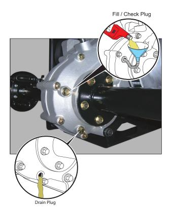
Clean the area around the check and fill plugs. Remove the check plug. The correct lubricant level is **just** below the bottom of the threaded hole. If lubricant is to be added, remove the fill plug and add lubricant using a funnel. Add lubricant slowly until lubricant starts to seep from the check plug hole. Install the check plug and the fill plug. In the event that the lubricant is to be replaced, a drain plug is provided at the bottom of the differential housing.
