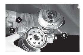
Oil capacity is 1 1/3 quarts (1.3 liters). Add slightly less than 1 1/3 quarts (1.3 liters) to allow for possible residual oil left in engine. The oil must be high quality oil that meets or exceeds API SF, SG, CC standards. Check oil level on dipstick. Oil should be slightly below 'H' to allow for expansion. If necessary, continue to add oil slowly and allow time for oil to flow down into engine. Check oil level on dipstick. **Do not overfill.**
