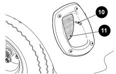
The only maintenance necessary for the first five years is the inspection of the rear axle for lubricant leakage. Unless leakage is visible, the lubricant needs to be replaced after five years. Refer to the Service and Repair Manual for the fluid replacement procedure.
